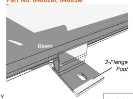
• **2-Flange Foot Material:** One of the following mill finished extruded aluminum alloys: 6005-T5, 6105-T5, 6061-T6
