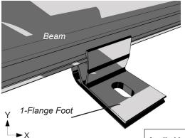
• **1-Flange Foot Material:** One of the following mill finished extruded aluminum alloys: 6005-T5, 6105-T5, 6061-T6
