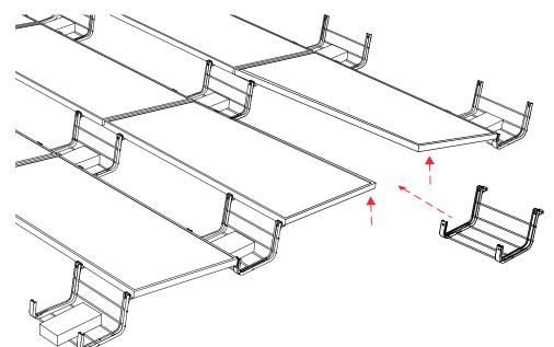
Apply gentle, even uplift on the two adjoining module frames, and slide bay into place.
