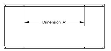
MEASURE DIMENSION (A) ON THE SOLAR PANEL TO DETERMINE WHETHER THIS SMALL SP BUCKET MOUNT WILL WORK IN AN OVER THE TOP OF POLE CONFIGURATION..
