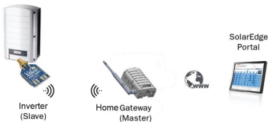
Figure 2: Connection to the SolarEdge Inverter
