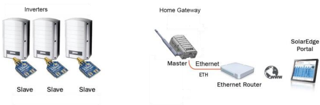
Figure 3: Connection to a Multiple Inverter Wireless Bus
