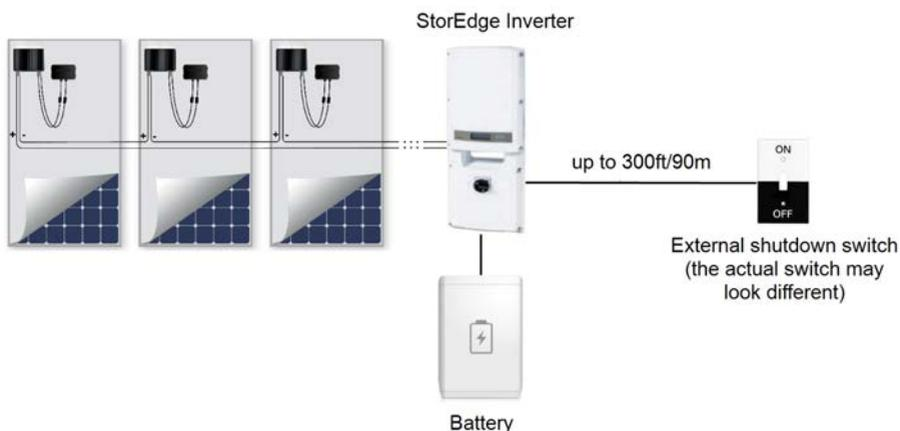
Figure 49: System connected to an external shutdown switch
