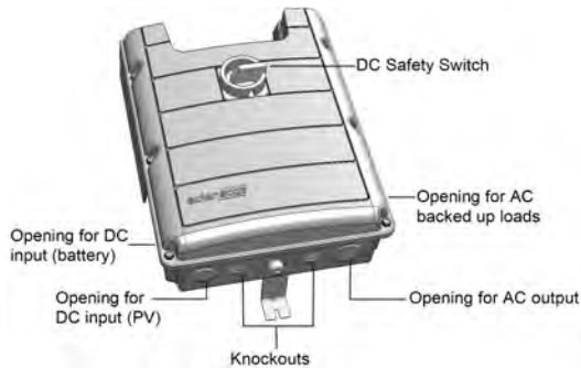
Figure 10: StorEdge Connection Unit
