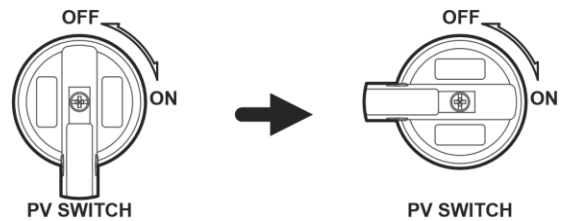
Figure 17: PV Disconnect Operation
