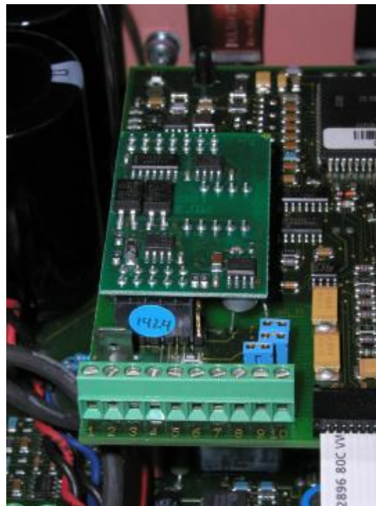
RS485 Board Installation
