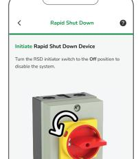
Figure 34 RSD verification in eSetup
