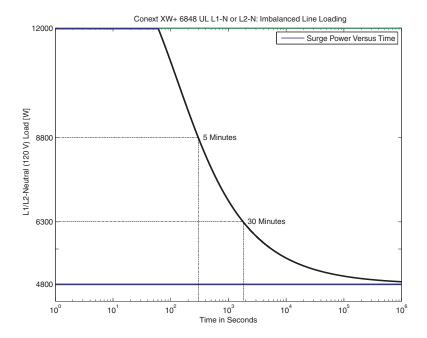
Figure A-1 Conext XW+ AC Overload Capability
