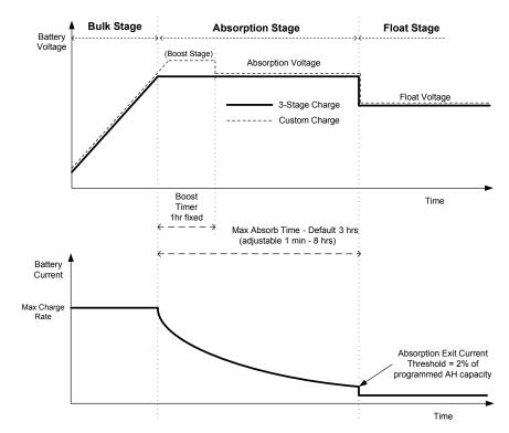
Figure 3-4 Three-Stage Battery Charging Cycle
