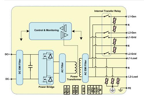
Figure A-6 Conext XW+ Block Diagram
