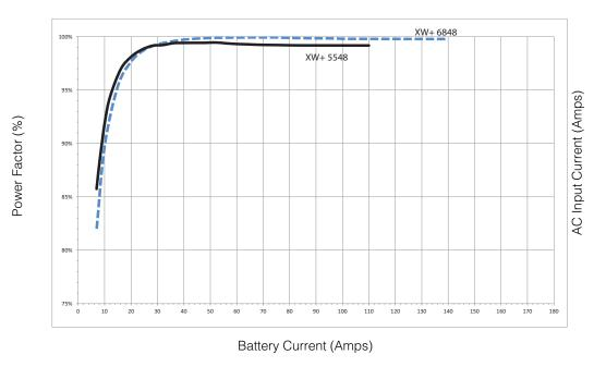
Figure A-5 Charging Efficiency (Power Factor)
