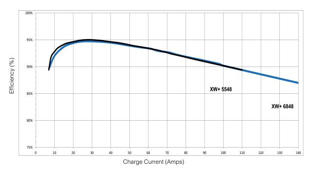
Figure A-4 Charging Efficiency (Typical)
