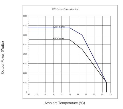
Figure A-2 Output Power Versus Ambient Temperature
