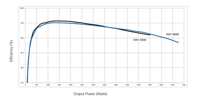
Figure A-3 Inverting Efficiency (Typical)
