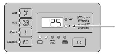
Figure 2-3 Inverter Information Panel When Charging Battery
