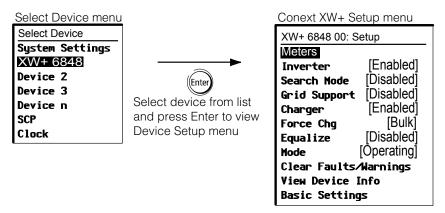
Figure 2-5 Selecting a Device Setup Menu
