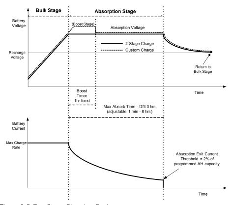
Figure 3-5 Two-Stage Charging Cycle
