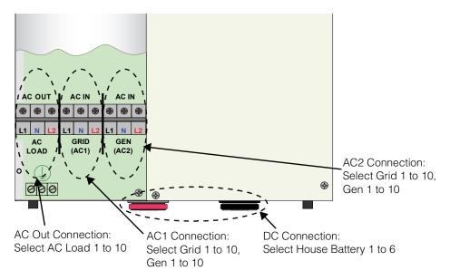
Figure 3-11 Conext XW+ Connections Representation
