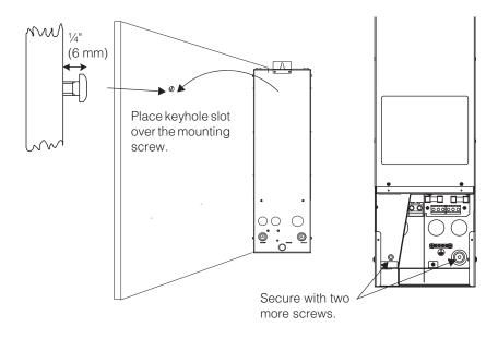
**NOTE**: When choosing a wall to install the solar charge controller, choose a wall that is not considered a flammable material such as concrete, brick, or metal.
