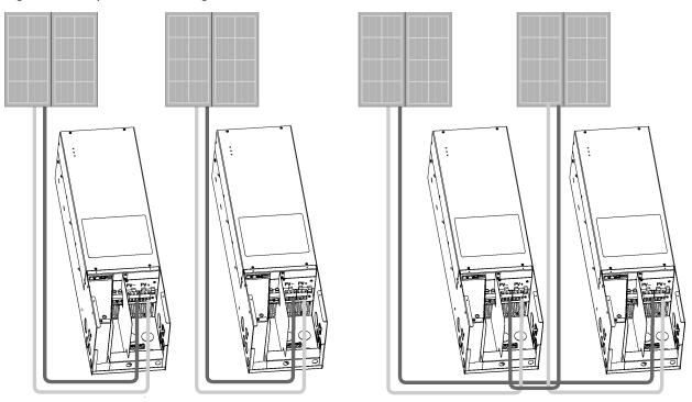
**Left:** Correct wiring —no interconnection between systems
