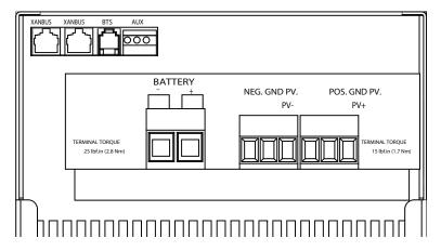
A label providing details on each connector and torque requirements for each terminal is affixed to the inside of the wiring compartment cover plate.
