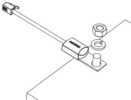
3. Route the sensor cable to the charger and plug it into the Bank 1 (default if using only one BTS), Bank 2 or Bank 3 connector on the rear panel. It may be advantageous to temporarily apply a layer of tape around the connector to protect its locking tab from catching on something during pulling and routing.
