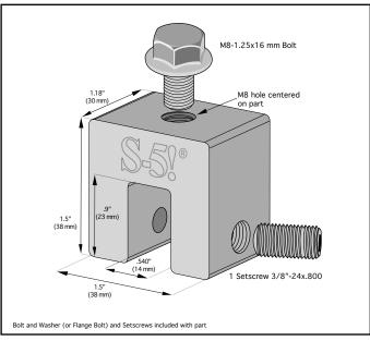
The S-5-S and S-5-S Mini clamps are each furnished with the hardware shown above. Each box also includes a bit tip for tightening setscrews using an electric screw gun. A structural aluminum attachment clamp, the S-5-S is compatible with most common metal roofing materials excluding copper. All included hardware is stainless steel. Please visit www.S-5.com for more information including CAD details, metallurgical compatibilities and specifications.
