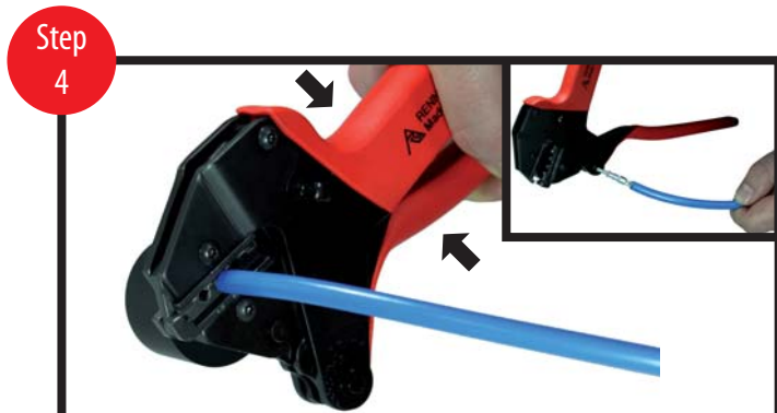
Position stripped end in the terminal, COMPRESS THE HANDLES UNTIL THE RATCHET AUTOMATICALLY RELEASES. CRIMPING PROCESS IS COMPLETED.
