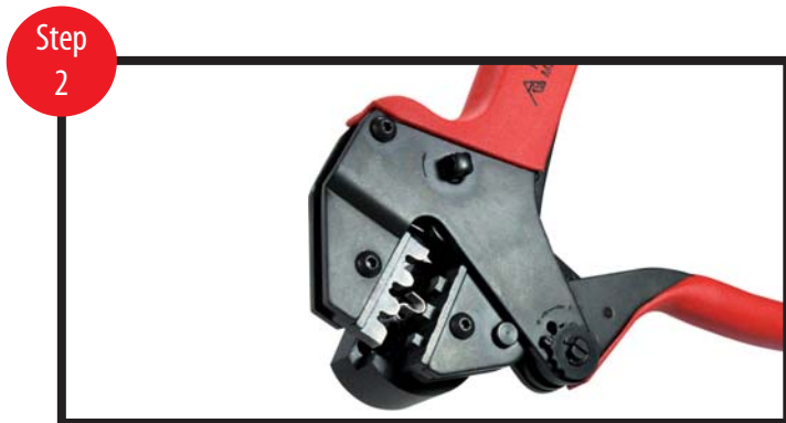
Hold tool so that the terminal can drop into the locator round hole. Make sure terminal is fully seated in the locator.
