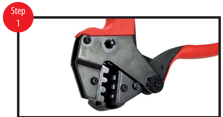
Compress handles until dies open. Select cable size as shown on top of crimp plate.
