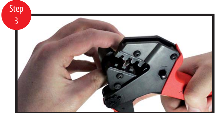
If necessary use your fingers for assistance to prevent the terminal from twisting.
