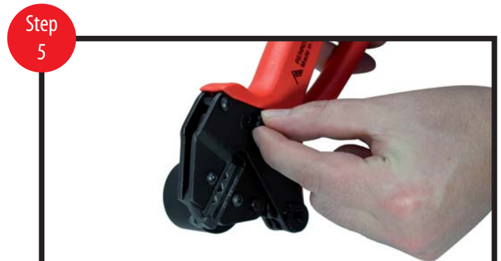
If jam occurs slightly compress handle while using fingers to rotate release clock wise.
