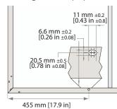
**Part Name** Specification Material Rail 6105 - T5 aluminum extrusion 1/4" x 20 - 5/8" ASTM F593 (stainless steel) Bolt 1/4" x 20 ASTM F593 (stainless steel) Nut
