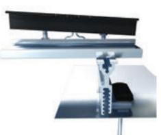
The bolt head underneath the clamp lines up and slides into the channel on the top of the slider of the base mount. At a module intersection that aligns with a rafter and mount location, engage either one of the bolts of the 8" panel clamp by pressing down the top clamp above the bolt, line up and slide into the channel on the top of the slider.
