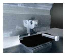
You can install the grounding lug at any time after the base mounts are installed. The system only requires one Ilsco GBL-4DBT grounding lug. Replace the cap screw in any base mount top slider with grounding lug hardware. Secure your wire to the lug by tightening the set screw. See full **Quick Rack Installation Manual** for system grounding specs and information.
