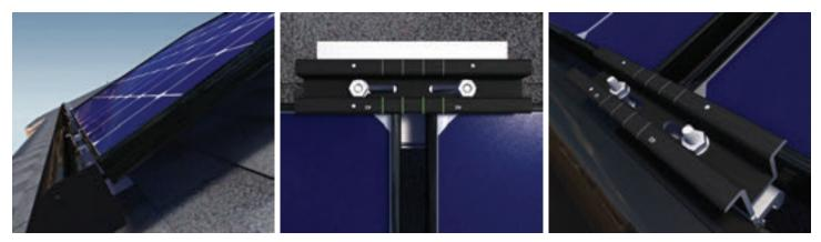
Insert the bottom edge of the module frame into the lower clamps. The top of the module sits on the lower portion of the clamp assembly for the row above.
