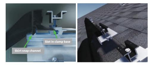
Insert horizontal leg of the skirt into slot in clamp base, then snap the skirt down in skirt snap channel. Slide instead of snap the floating 8" bridge clamps halfway onto end of the skirt segments at the module intersections then slide the next segment onto the other side of the clamp making segments flush.
