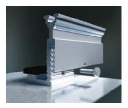
To adjust top slider height, remove machine bolt, separate top slider from QBlock slider and reinsert at proper location. To adjust in ¼" increments move the top slider up or down one notch. To adjust in ½" increments rotate the top slider 180 degrees. Repeat for the other mounts until top slider elevations are uniform across the row.
