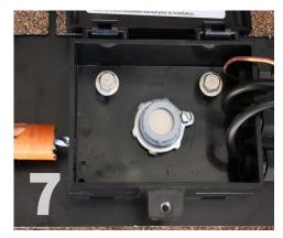
Holes for Conduit: Use the drill starter along the perimeter of the box to guide your hole saw specified by the conduit hub manufacturer. Clean off all burs. Attach the conduit to the box. Ensure that conduit cap and blank are installed.
