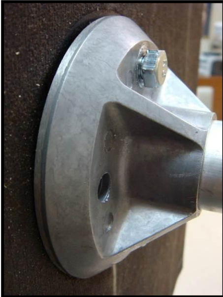
Figure 3. Lag Bolt Pull-Out Shear Parallel to Rafter
