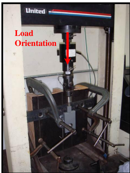
Figure 1a. Shear Parallel to Rafter
