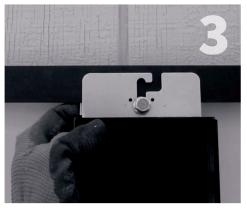
Slide this assembly onto the module frame with the bracket behind the module frame, the module level electronic mounting bracket in front of the module frame.
