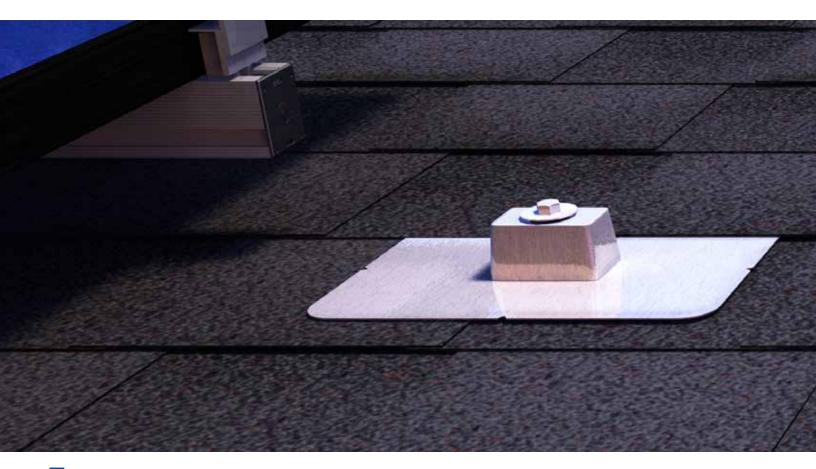
he Classic Composition Mount and the E-Mount series are designed for fast, simple installation onto existing composition/asphalt shingle roofs. Both mounts use Quick Mount PV's QBlock Elevated Water Seal Technology® for a long, watertight life on the roof. Both series are also available with multiple attachment options: lag bolt, hanger bolt and extended hanger bolt.
