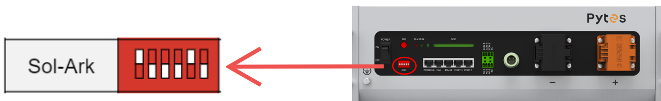
Figure 2.1.1.4 Sol-Ark inverter DIP Switch Setting
