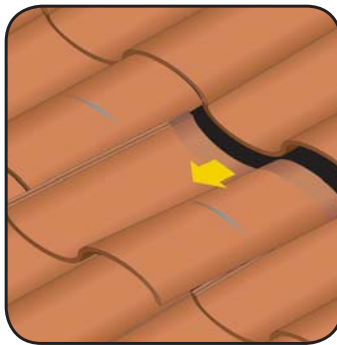
STEP 2: Remove the tile by pushing and pulling. It is usually held in place by a small nail.
