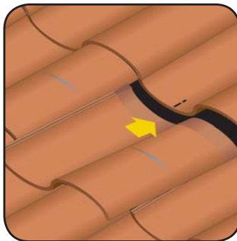
Step 8: Replace the tile by lining up the snap lines and mark the drill location accordingly.
