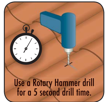
Step 9: Using a 1/2" carbide drill bit and ROTARY HAMMER DRILL in hammer mode, drill through the tile. See online video at www.prosolar.com for details.
