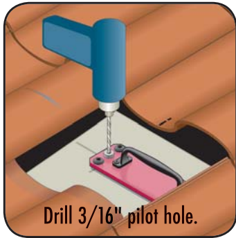
Step 4: Seal the initial tile nail hole. Using a 3/16" drill bit and drill guide (FJ-Drill), drill pilot hole along the rafter center
