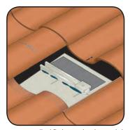
Step 8: Install subflashing and seal as needed if double flash is desired.
