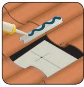
Step 5: Insert the lag bolt and washer through the TileTrac® and apply fresh compatible sealant to the base.
