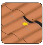
Step 9: Replace the tile by lining up the snap lines and mark the drill location accordingly.
