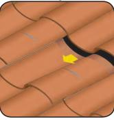
STEP 2: Remove the tile by pushing and pulling. It is usually held in place by a small nail.
