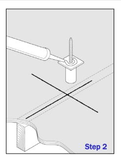
STEP 2: Apply a generous amount of roof sealant to the bottom of the seal plate of the SolarWedge<sup>®</sup> XD creating a circle around the lag bolt hole.
