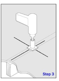
STEP 3: Using a cordless impact wrench and a 9/16" deep socket, install the bolt into the Solar-Wedge® XD base until seated. Allow the sealant to flow outward around the edges of the seal plate.
