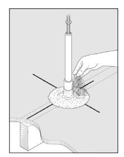
**STEP 6:** Using Play/Silica sand, cover the sealant. *This step prevents debris from sticking to the sealant while drying and gives it a clean, finished appearance.* **IMPORTANT: Do not install leveling** *kit hardware until support rail installation.*
