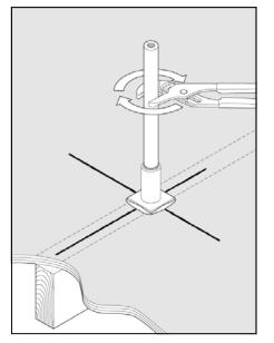
STEP 4: Install the post using an adjustable wrench. Turn wrench clockwise until fully secured. Avoid twisting the base while tightening.
