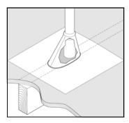
**Flash** The SolarWedge® is compatible with readily available, standard 1" roof flashings.
