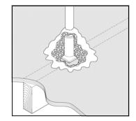
Foam Using a 2-part hand-held or truck mounted foaming rig, you can create a "flashing" using high density roof foam!
