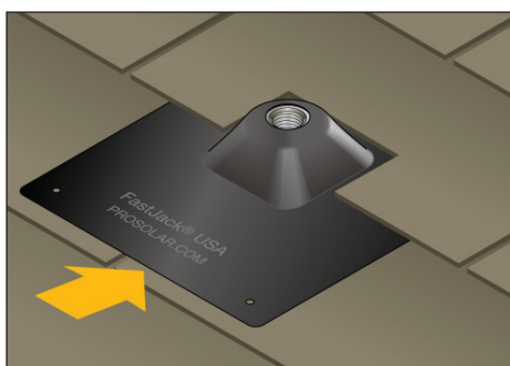
Step 5: Slide FastJack® flashing under shingle
