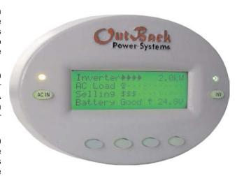
The OutBack MATE also includes a built in real time clock and calendar which allows programming of the inverter operation based on the time of day and even day of the week. This can be used to allow the system to work with time-of-day power rates or to limit a generator's run time to a specific time period of the day or week.
