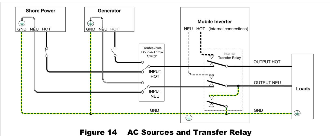
**Figure 14 AC Sources and Transfer Relay**
