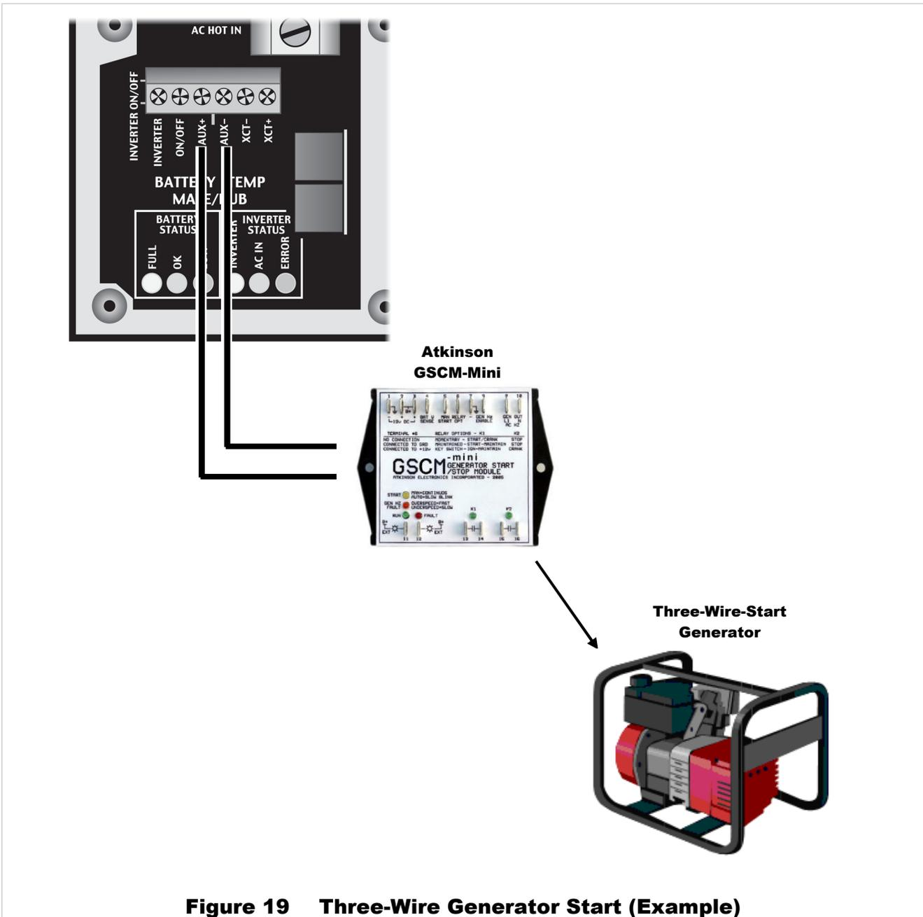
**Figure 19 Three-Wire Generator Start (Example)**
