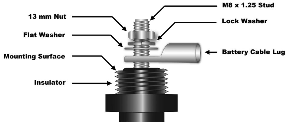
**Figure 8 Required Order of Battery Cable Hardware**
