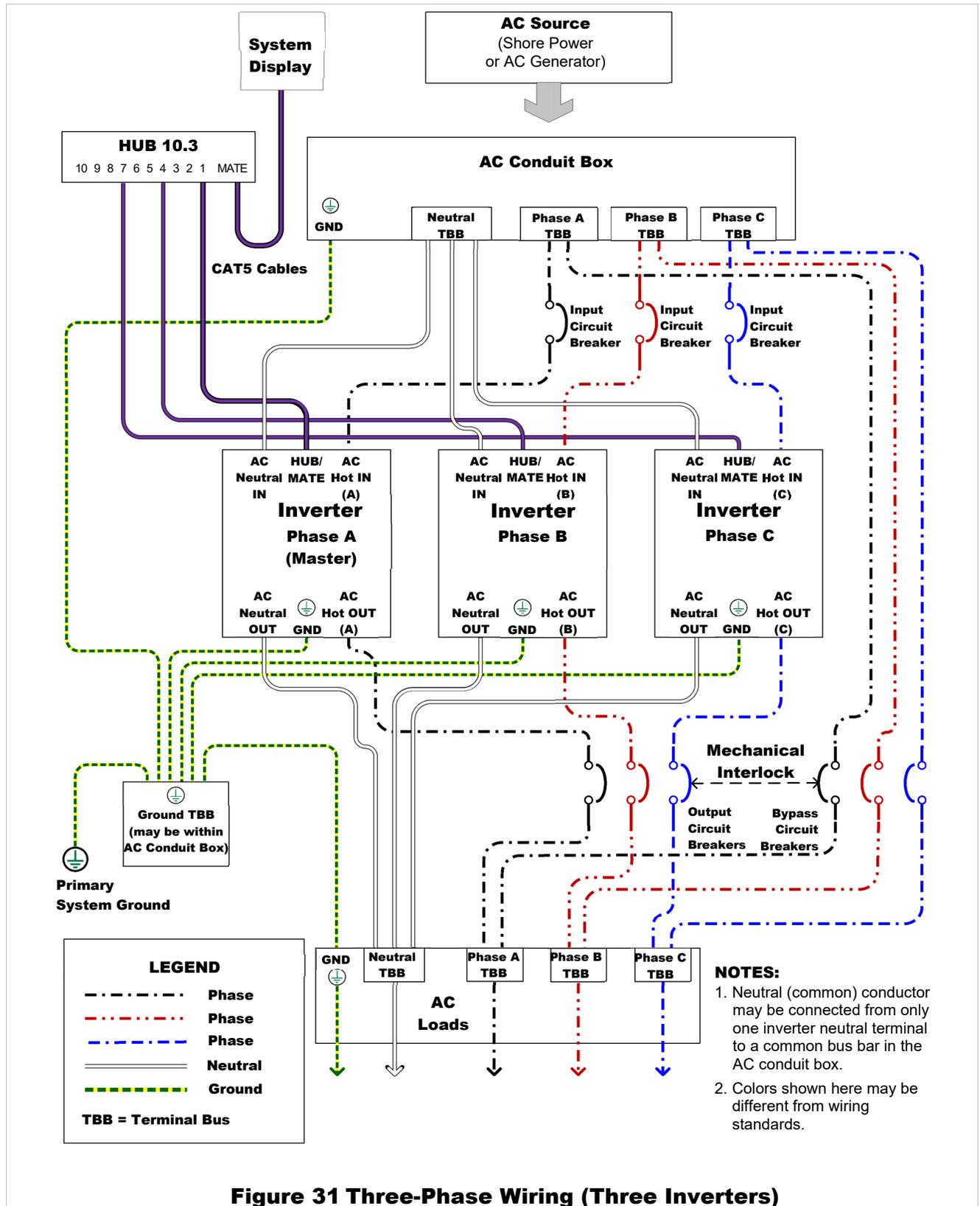
**Figure 31 Three-Phase Wiring (Three Inverters)**
