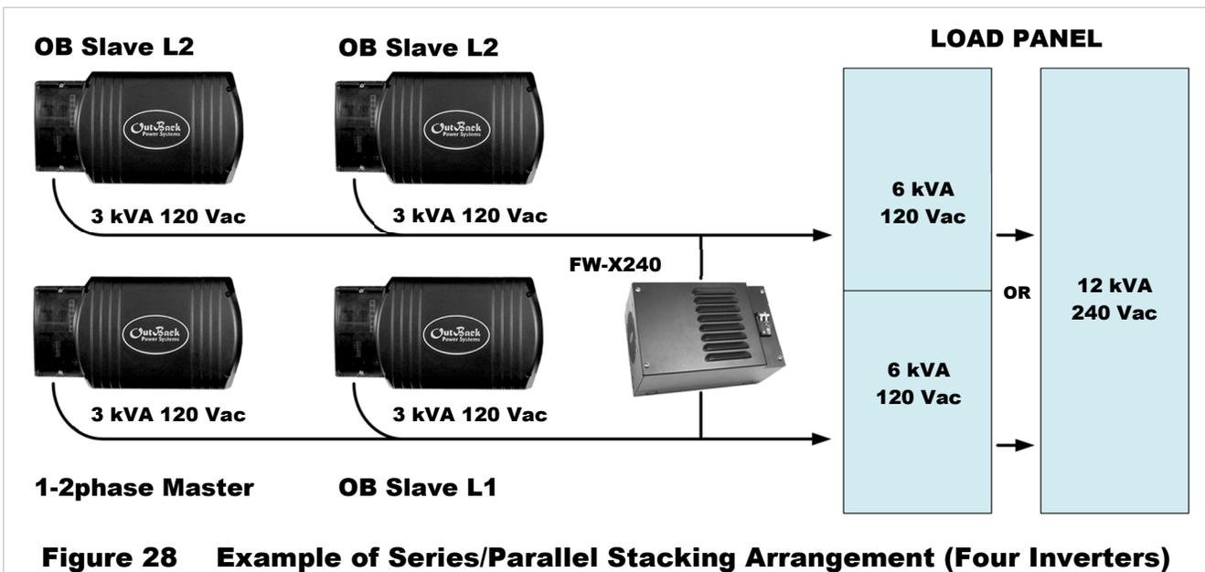
**Figure 28 Example of Series/Parallel Stacking Arrangement (Four Inverters)**
