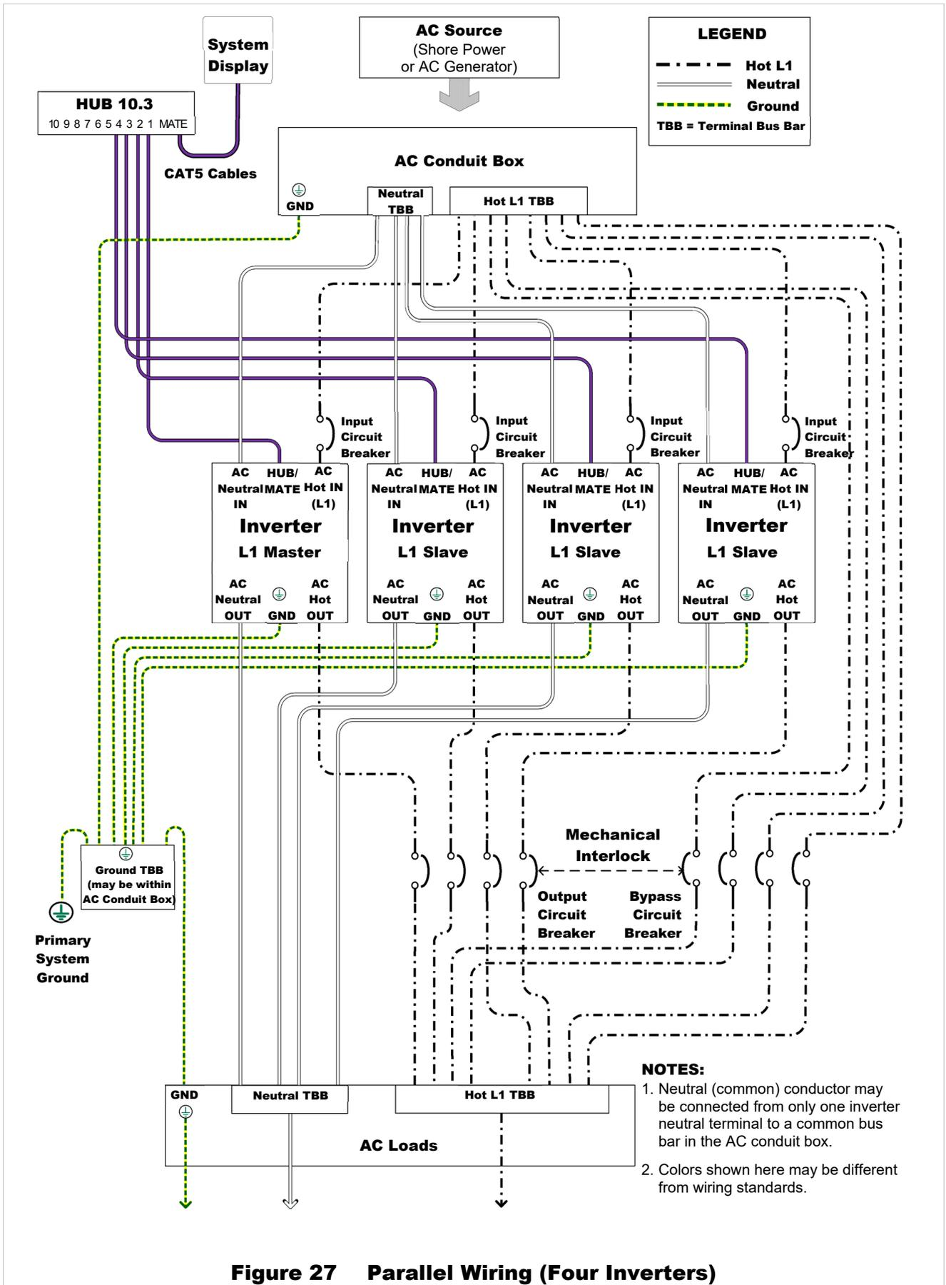
**Figure 27 Parallel Wiring (Four Inverters)**
