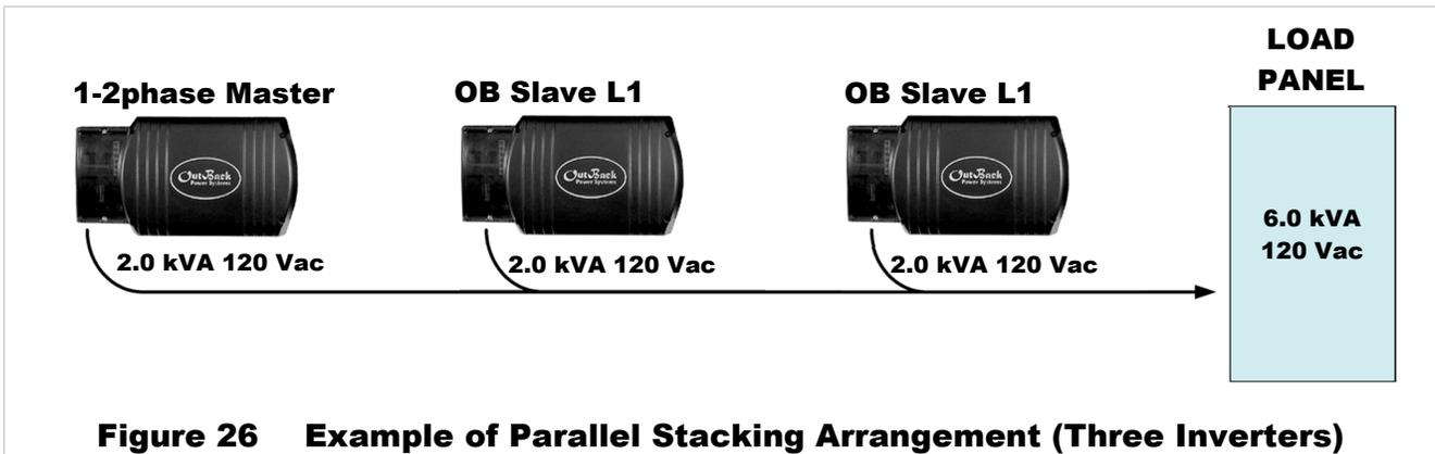
**Figure 26 Example of Parallel Stacking Arrangement (Three Inverters)**
