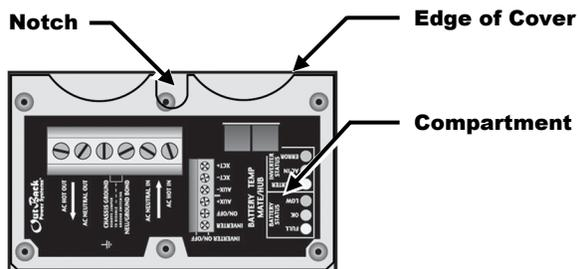
If necessary, the green terminal block can be unplugged by pulling it gently away from the AC board.
