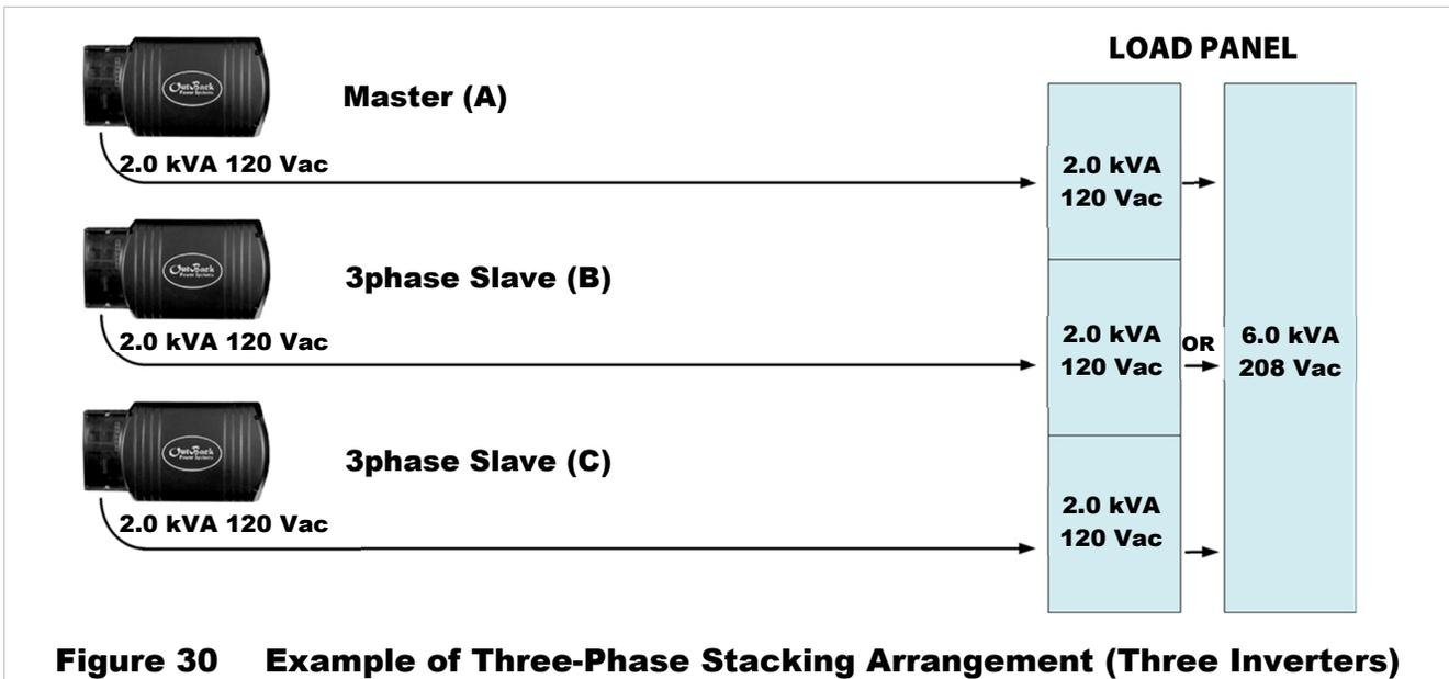
**Figure 30 Example of Three-Phase Stacking Arrangement (Three Inverters)**
