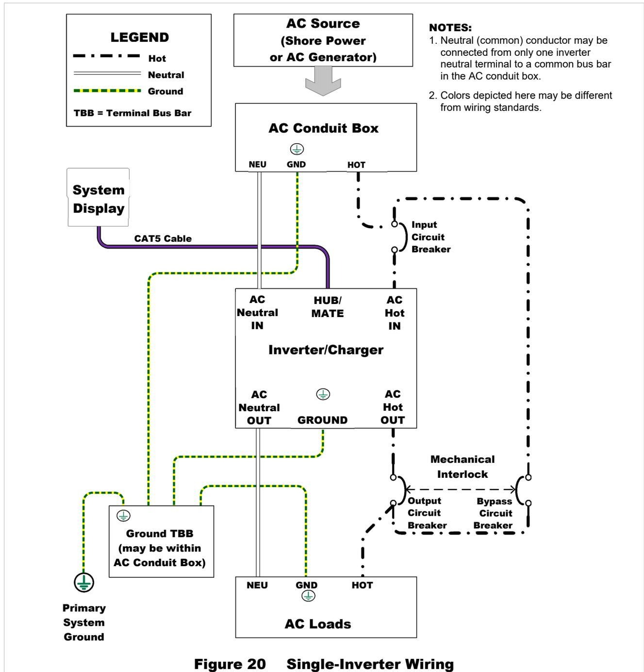
Figure 20 Single-Inverter Wiring
