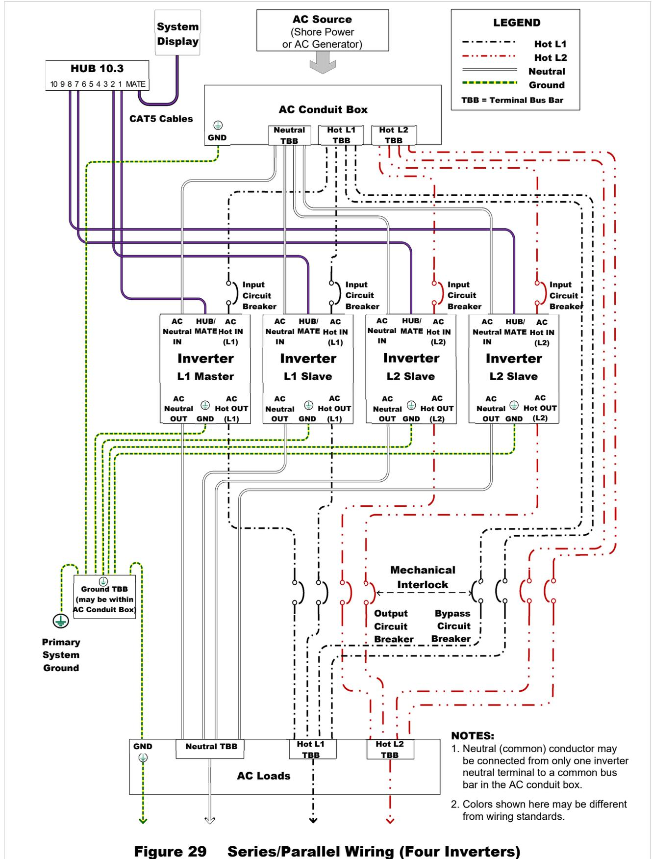
**Figure 29 Series/Parallel Wiring (Four Inverters)**
