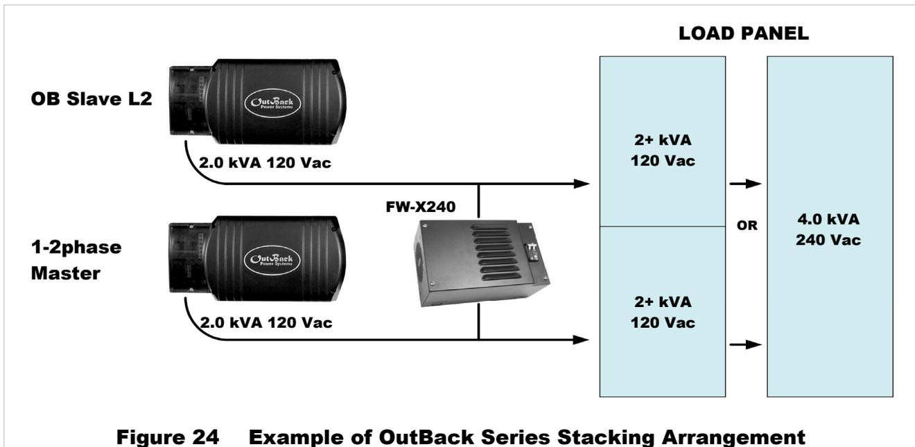
**Figure 24 Example of OutBack Series Stacking Arrangement**
