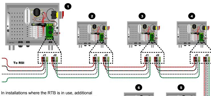
combiners require additional RTB devices. One RTB pole is required for rapid shutdown of each PV circuit. For six arrays, the recommended method is to use one PNL-75Q-DC-RT for shutdown of four arrays and one PNL-75D-DC-RT for the other two. The BKR-CTRL-DC can drive up to three RTB devices.
