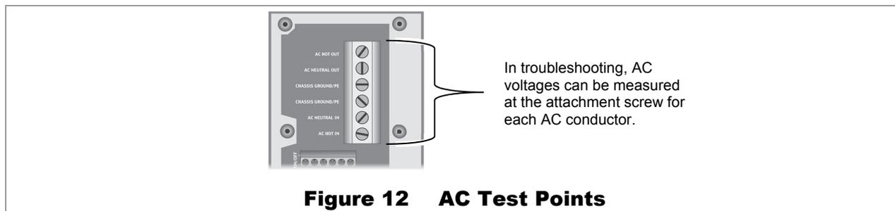
**Figure 12 AC Test Points**
