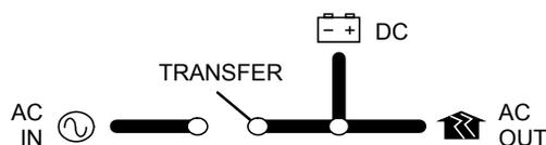
These items represent the input from the AC source, the output to the AC loads, DC functions (inverting, charging, etc.), and the transfer relay. Arrows on each symbol represent power flow.
