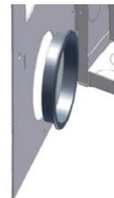
Figure 11, Installing 3.5" Grommet in the Door
