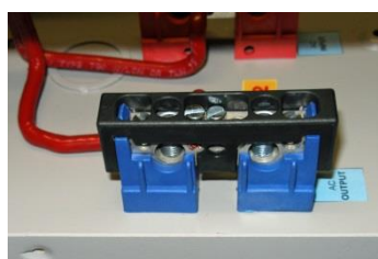
Replace wiring cover. Black cover shown here
