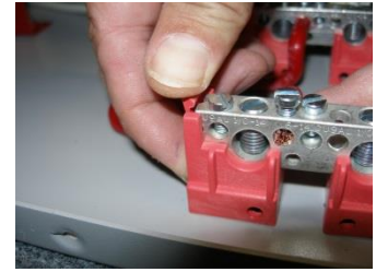
Gently pry back ear of mounting block and push up on terminal block from below
