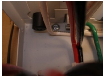
Chassis ground connection to inverter
