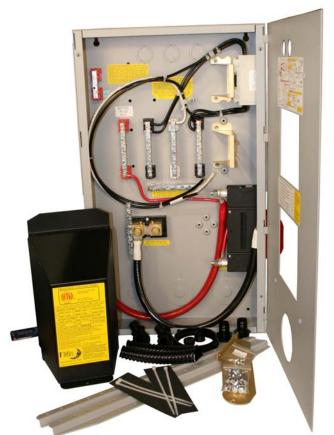
OB version for these professionals. It is based on the 50% wider Magnum Energy chassis. In addition to more room to work, you also get a PV input busbar, Battery Plus and DC negative busbar. No need for ring terminals anymore with this system! There are also additional knockouts top and bottom for lightning arrestors and cabling. Professionals feel the additional \$70 list price is well worth it.
