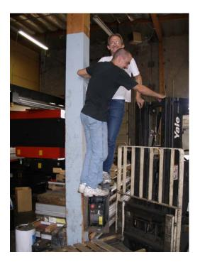
Yes, there are two guys standing on the door of an E-Panel with the door open and inverter installed. This was actually a UL required test of the hinged door.
