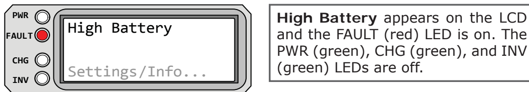
Figure 5-19, High Battery Fault
