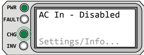
Figure 5-22, AC In – Disabled Mode
