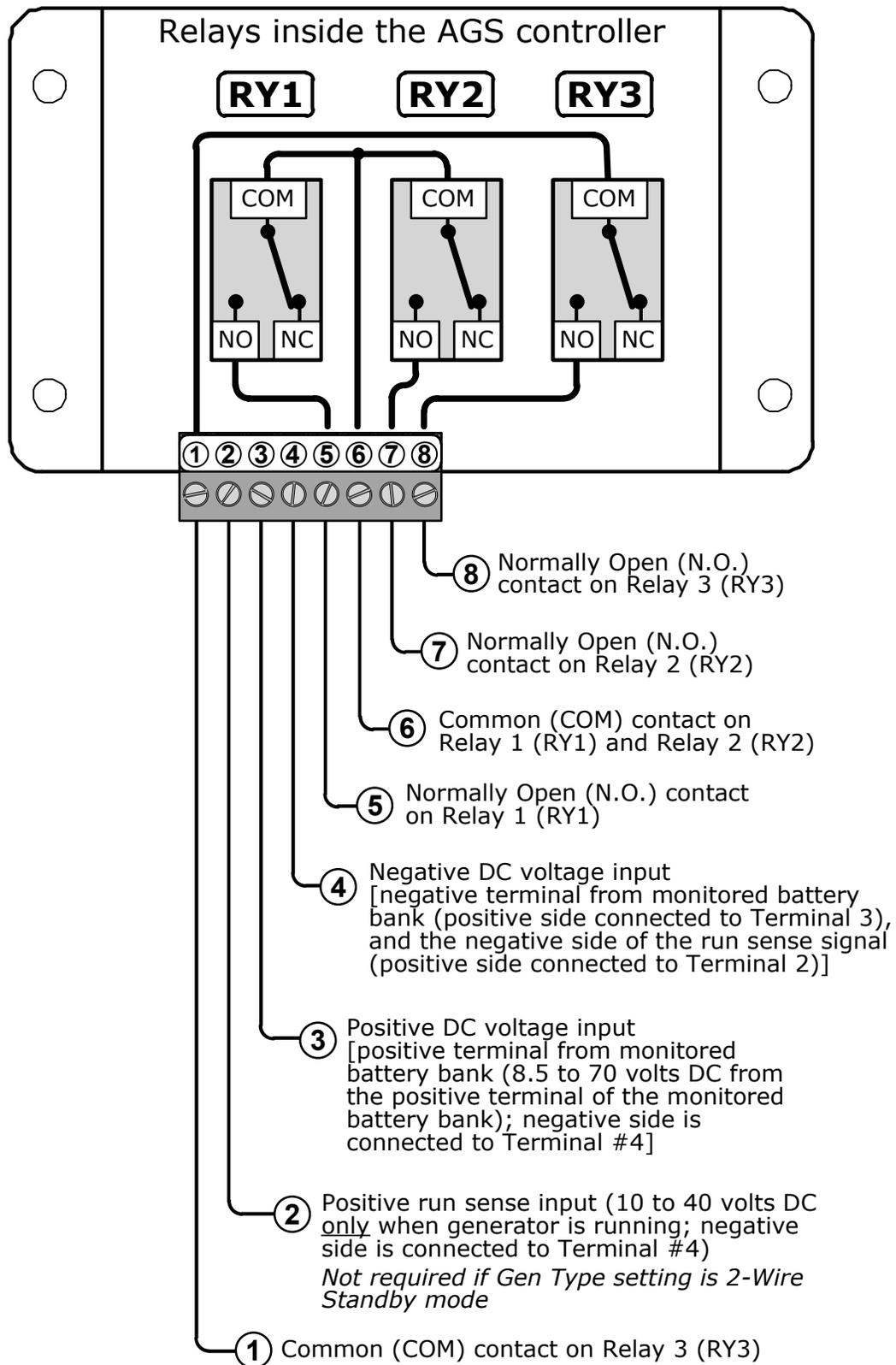
**Figure 2-11, Wiring to the ME-AGS-N Module's Terminal Block**
