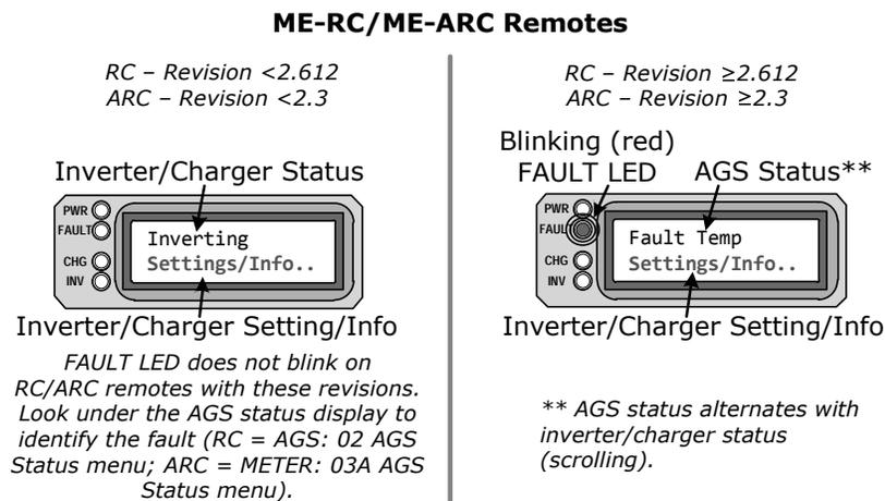
**Figure 12-1 ME-AGS-N Fault Message - RC and ARC Screens**
