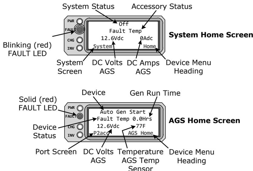
**Figure 12-2 ME-AGS-N Fault Message - Router Screens**
