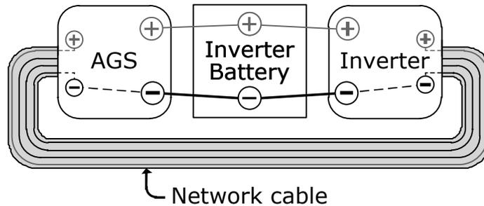
**Figure 2-9, Connected Devices at the Same Potential**
