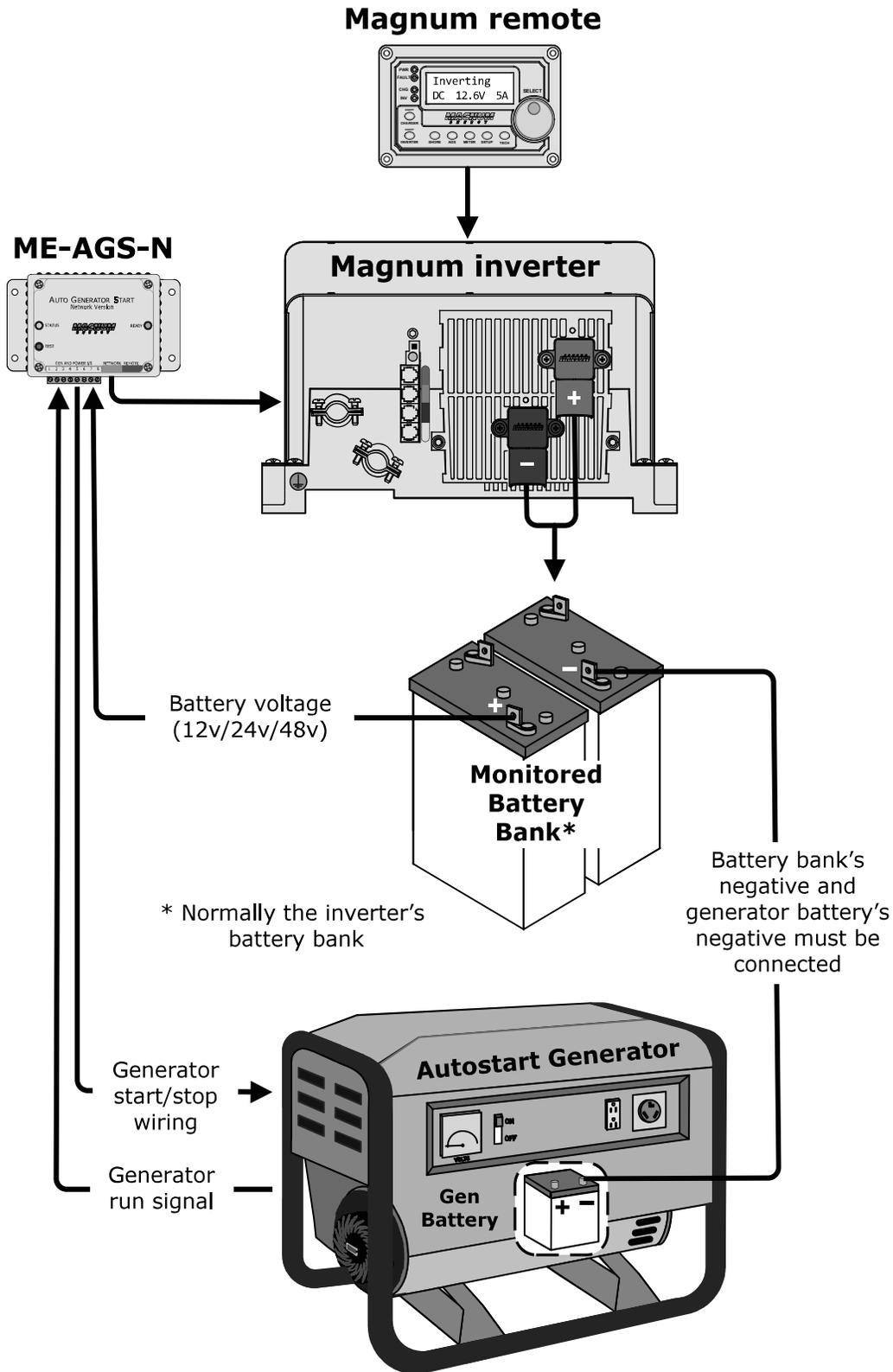
Figure 2-1, ME-AGS-N System Diagram
