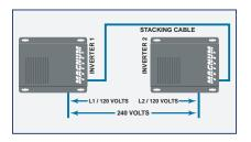
The Series Stacking Cable Kit allows two inverters to be stacked together to achieve 120/240 VAC output. Series stacking is commonly used for well pumps, tools, motors, and other 240 VAC appliances. The kit includes communication cable, two 2/0 battery cables, and battery lug covers.
