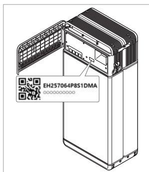
1. Battery Control Unit QR Code
