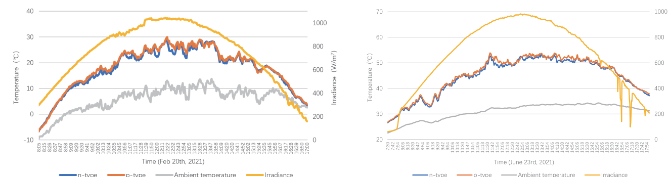
Figure 5 : Operational temperature comparison of n-type and p-type PERC modules
