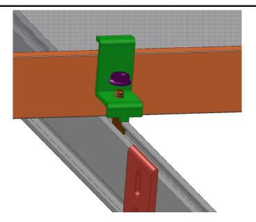
3. Complete the clamp assembly with a flange nut as shown.
