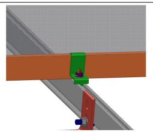
**5.** Working from the opposite side of the PV module. Assemble the center clamps by putting a clamp on the bolt, then the flange nut.
