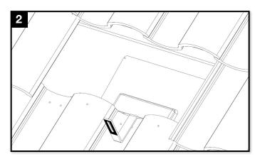
Position the flashing over the base of All Tile Hook so that the flashing completely covers the base.
