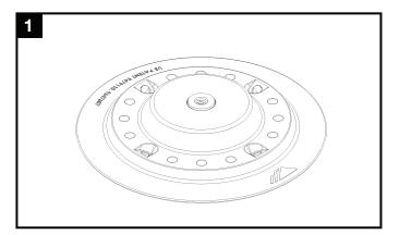
Mark locations for Flat Roof Attachment. Roof screws can be installed before or after racking is installed. Type, size, and quantity of roof screws to be specified by Structural Engineer. Fastener size not to exceed #15. Screws should be installed symmetrically to each other.
