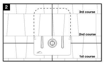
Slide flashing, between 1st and 2nd course, so the top is at least 3/4" above the edge of the 3rd course and the bottom is above the edge of the 1st course.
