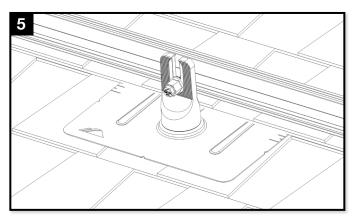
Attach rails to either side of the open slot using bonding hardware. Level rail at desired height, then torque to 250 in-lbs (21 ft-lbs).
