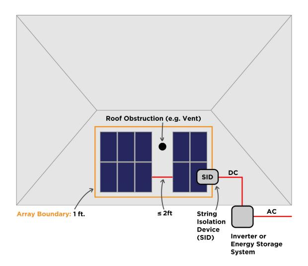
Case 2: Maintaining NEC Compliance with sub-array(s) within array boundary.
