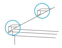
**Optional:** Using the included battery module fixing brackets (included in each battery module box) the battery modules within the stack can be fastened together for even greater stability. You will need to remove the other side panel on each battery module to access these attachment points. You will also need to remove the top panel of the BMS and the other side panel of the BMS to gain access to the top attachment point. (Doing so will not void the warranty)
