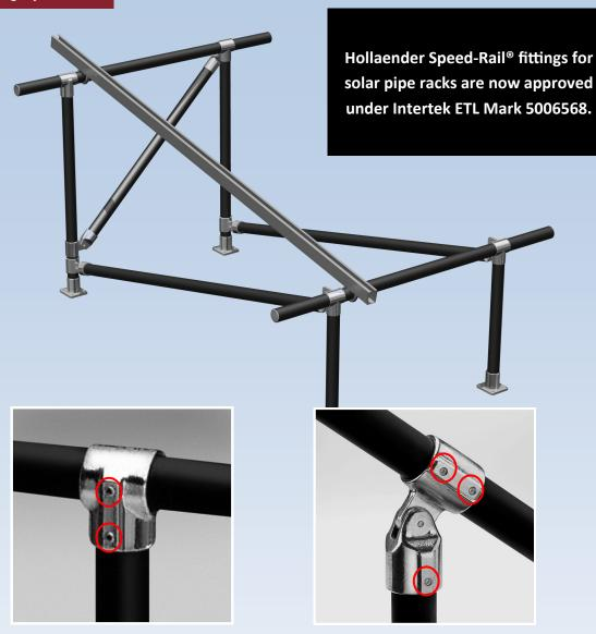
When properly installed, the set screws are electrically bonded to the pipe and bracing, thereby fulfilling the grounding and bonding requirements of UL 2703. This eliminates the need for additional bonding components.
