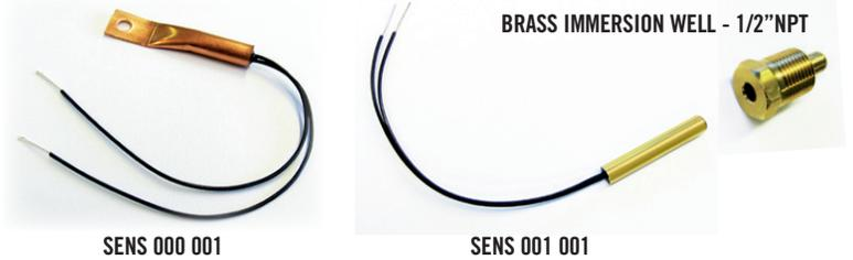
The sensor leads are 24AWG Class II and carry 4VDC. Use 18-24AWG zip or bell wire to run from the sensor location to the controller. Use caution when installing to avoid wire damage. Shielded wire is not necessary. Use insulation and weatherproofing for accurate sensor readings. Install out of direct sunlight.
