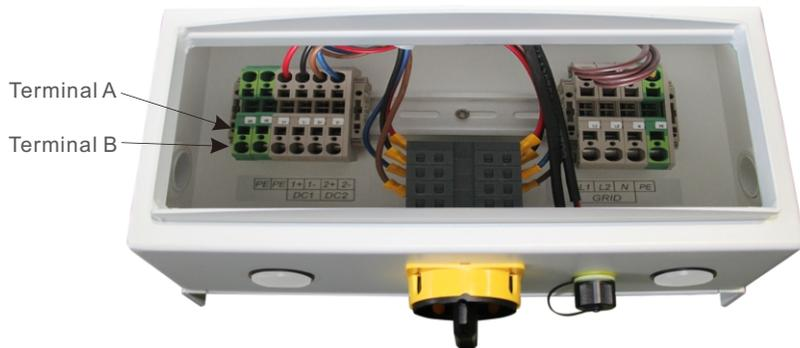
▲ Figure 4.6 Connection area of inverter(Non-Fuse type)
