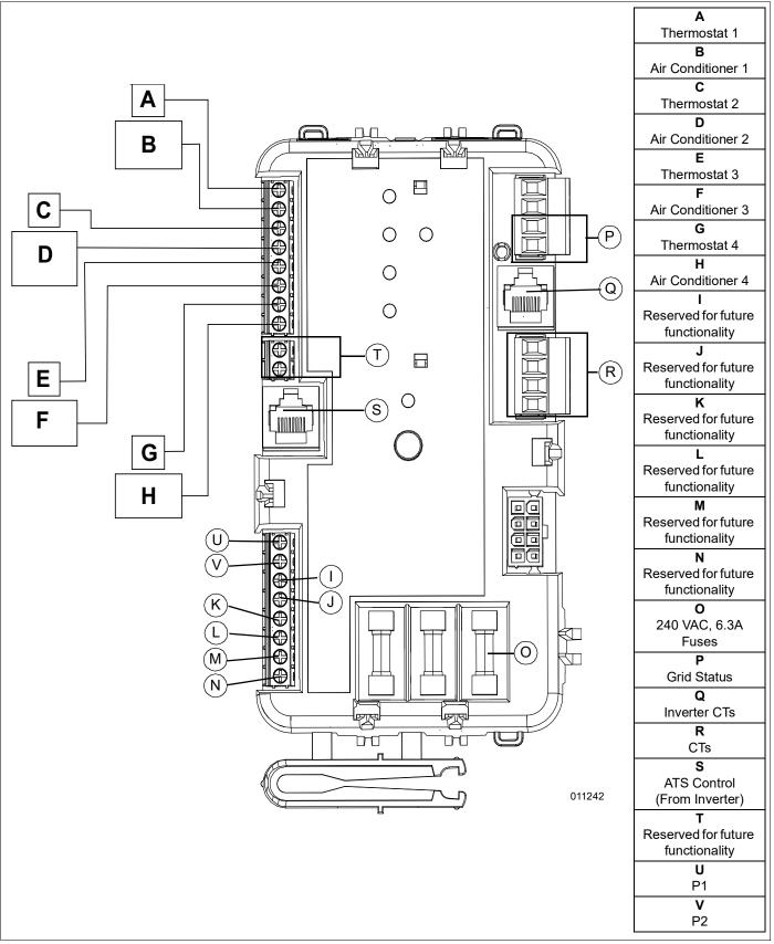
Figure 3-4. Controller Connections
