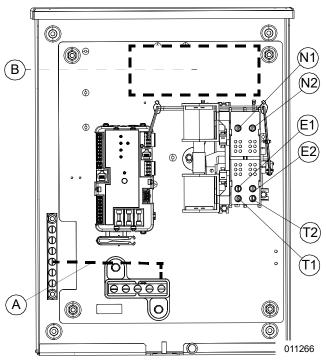
Figure 3-3. Wiring Connections 100 A Unit
