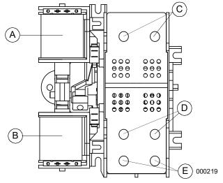
Figure 2-1. Typical Single-Phase ATS Transfer Mechanism
