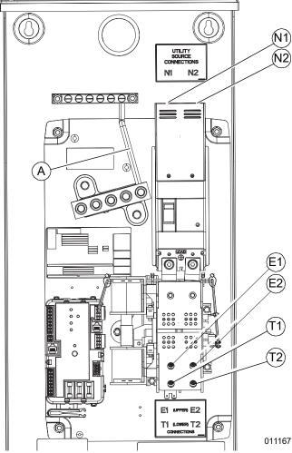
Figure 3-2. Wiring Connections 200 A Unit
