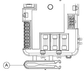
Figure 4-2. Fuse Removal and Installation Tool
