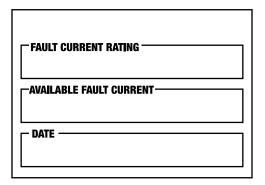
Figure 3-8. Fault Current Label
