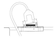
**b.** Cover any unused connectors with sealing caps. Listen for two clicks as the connectors engage. **See notes in** *Step Details* **on back.**
